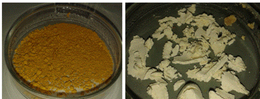
Figure 6. Hesperidin crude and after purification
