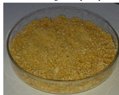
Figure 7. Dry waste material after extraction of oil, \beta -carotene and hesperidine.
